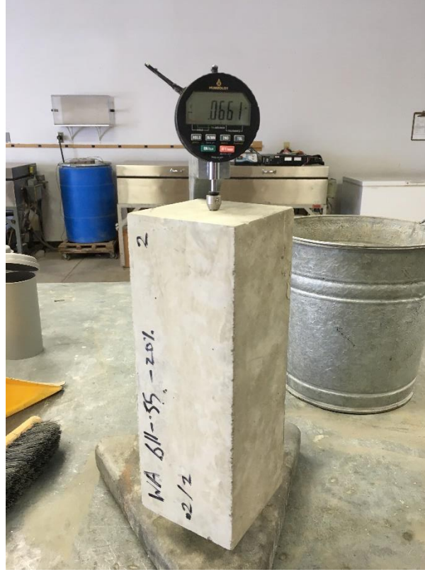
Figure 3.3. Prism resting in shrinkage apparatus
