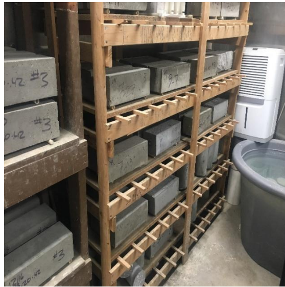
Figure 3.1. Drying Shrinkage specimens
