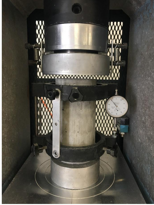
Figure 3.5. Modulus of elasticity setup using Forney
